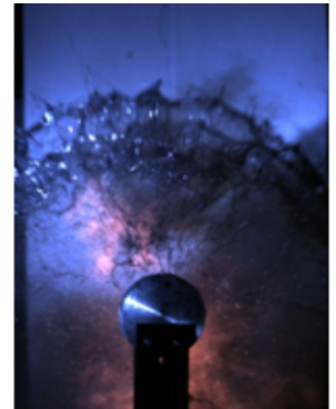
Fig. 4 Explosion-induced dispersal photos of liquid with different viscosity at the different times after explosive explosion
