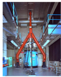
(b) AMS vertical ballistic range [56]
