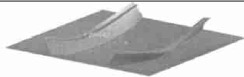
图 6 加筋板残余变形的计算结果 Fig. 6 The computational result of plate structure's residual deformation
