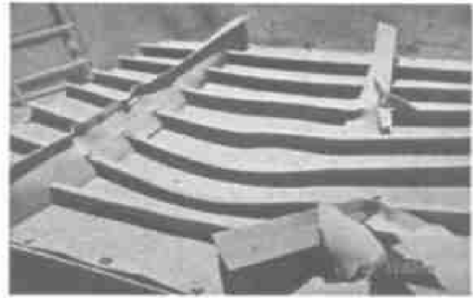
图 2 试验板架的残余变形 Fig.2 The experimental plate structure's residual deformation
