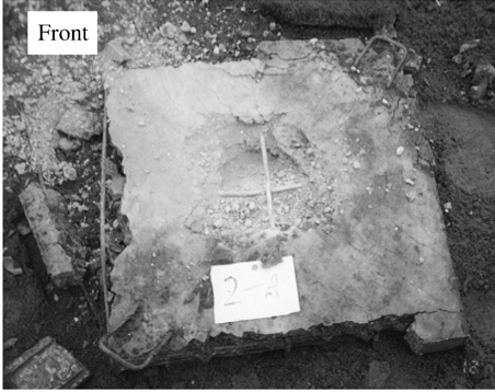
(b) Steel fiber reinforced concrete specimen
