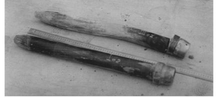
图 9 动能弹斜侵彻混凝土靶后弯曲变形 Fig. 9 Bending deformation of anti-runway KE projectile after oblique penetration
