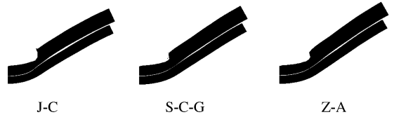
图 4 数值模拟的典型实验试件变形 Fig. 4 Computed deformations of samples in the typical experiment
