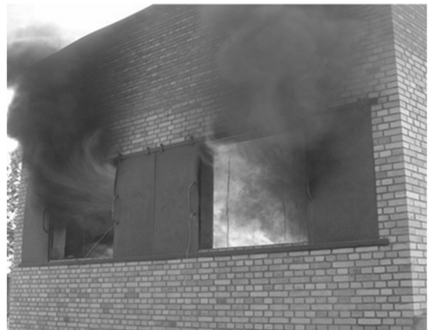
图9 大规模实验火灾中强轰燃实拍照片 Fig. 9 Practical photo of strong flashover in large-scale experimental fires
