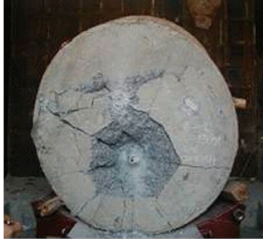
图 3 弹丸侵彻混凝土靶板的破坏情况 Fig. 3 Damage of concrete target penetrated by projectile
