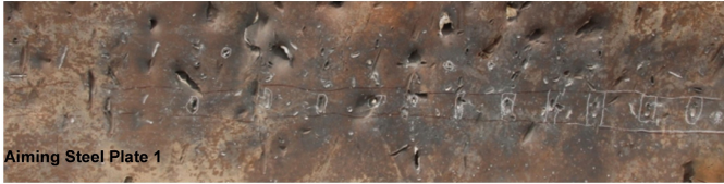
(c) Detail of damage at steel plate for test 1
