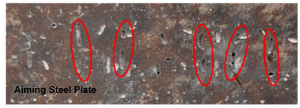
(d) Detail of damage at steel plate for test 2
