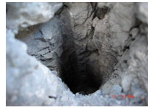
图3 刻槽弹体侵彻混凝土隧道区洞口外形 Fig. 3 Hole formed in the tunnel stage
