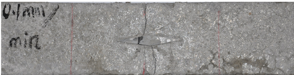
图6 慢速加载试件破坏形态图 Fig. 6 Failure maps at a low loading rate
