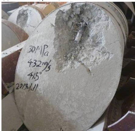
(c) v=432 m/s, \beta=42^\circ , no ricochet
