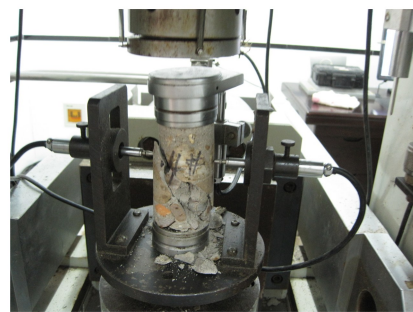
图 1 相似材料配比试件强度实验 Fig. 1 Strength experiment of samples with similar material ratios
