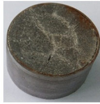
(b) 20 \text{ }^{\circ}\text{C} , \dot{\epsilon}=122 \text{ s}^{-1}
