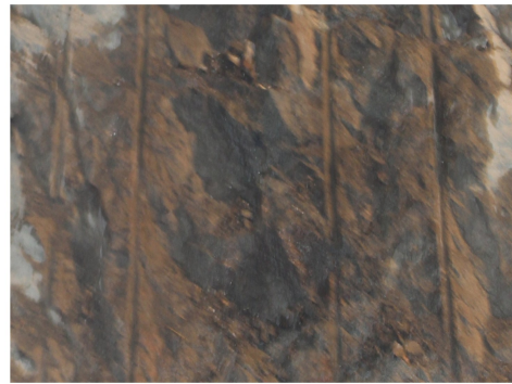
图10 后爆孔为 70\text{ cm} 的爆破效果图 Fig. 10 Blasting effect (observed when the distance between the later detonated holes is 70\text{ cm} )
