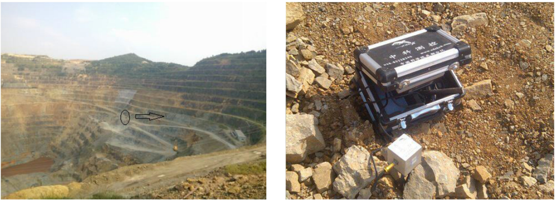
图 7 爆破振动速度现场监测 Fig. 7 Field monitoring of blasting vibration velocity
