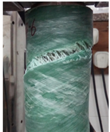
图 4 玻璃纤维增强型复合材料轴向拉伸断口 Fig. 4 Fracture appearance of GFR composite material specimen in overall tensile experiment
