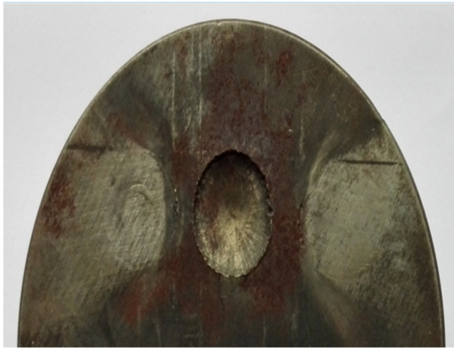
图 6 实验距离 6 和 8 mm 见证块凹坑 Fig. 6 Deformation of steel witness plate at 6 and 8 mm
