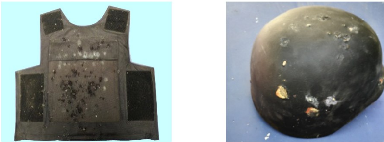
图 5 防弹衣与防弹头盔(试验后) Fig. 5 Bulletproof vest and helmet (after the experiment)
