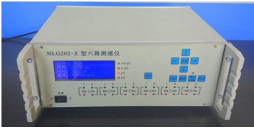
图 3 NLG202-Z 型六路测速仪 Fig. 3 NLG202-Z tachometer
