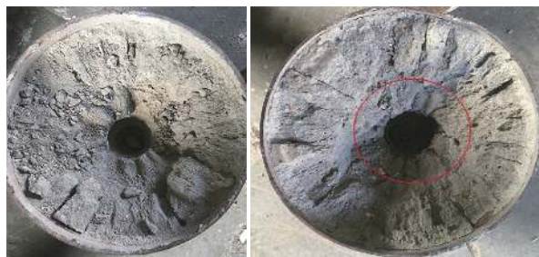
(a) Model of columnar explosive charge (b) Model of shaped charge in spiral tube
