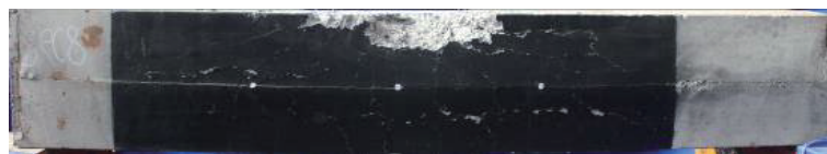
(c) Specimen SRC9 ( v=9.39 m/s, E=51.08 kJ)
