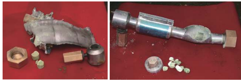
Recovery tube wall and explosive in thin wall DDT experiments
