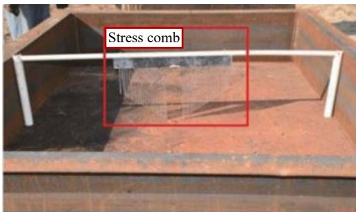
图 6 应变梳布置 Fig. 6 Strain comb arrangement
