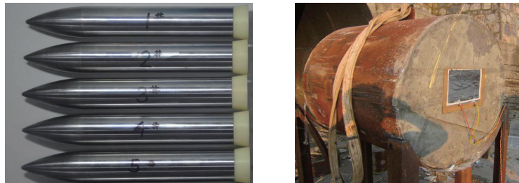
图 4 实验弹靶 Fig. 4 Projectile and target used in penetration experiments
