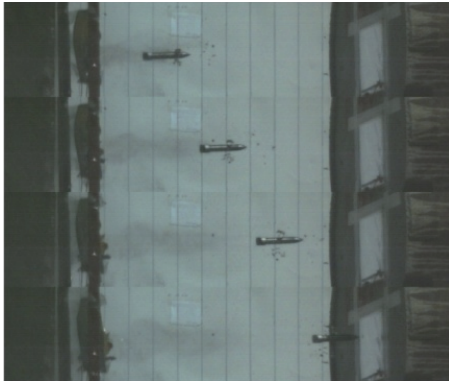
图 5 高速摄影记录的弹体撞击靶体过程 Fig. 5 Process of projectile impacting target recorded by high speed photography
