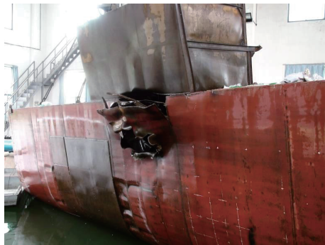
图 16 舰船结构缩比模型内部爆炸破坏 [81] Fig. 16 Damage of the scaled ship structural model by internal explosion [81]
