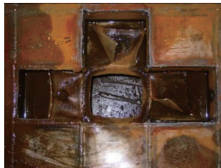
图 17 多箱型结构“十”形破坏效果 [81] Fig. 17 Cross-shaped damage effect of a multi-box structure [81]
