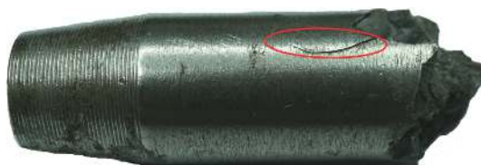
图 7 残余弹体出现的裂纹 Fig. 7 A large fragment with a crack on the side
