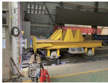
(a) Collision test system for railway vehicle components in Central South University
