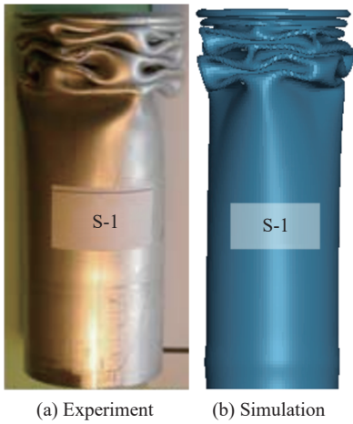
图 4 S-1 模型实验与数值模拟变形模式对比 Fig. 4 Comparison of experiment and simulation deformation modes of S-1 model
