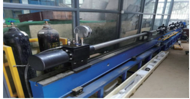
图 2 SHPB 系统及同步智能箱式电阻炉 Fig. 2 SHPB system and synchronous intelligent box-type resistance furnace
