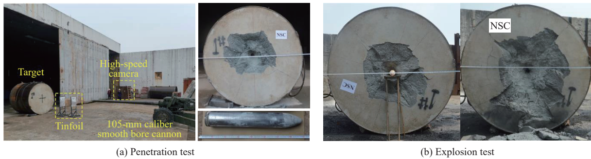
图 7 侵彻爆炸联合作用试验 Fig. 7 Combined penetration and explosion test
