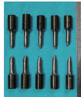
Fig. 2 Static stress-strain curves of smooth round bars under different strain rates and specimens with tensile fracture
