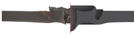
图 16 非偏心环锥罩的试验结果和数值模拟结果对比 Fig. 16 Comparison between experimental and numerical simulation results of non-eccentric liner
