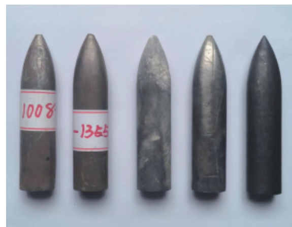
图 7 回收到的 4 发弹体(左 1~4)和原始弹体(右 1) Fig. 7 The recovered four residual projectiles (1st to 4th from left) and original projectile (1st from right)
