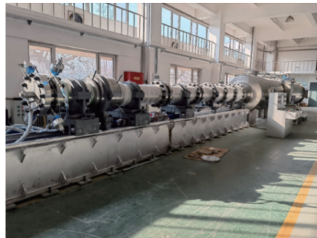
图 9 近场爆炸冲击波模拟激波管装置 Fig. 9 The shock tube device for simulating near-field blast wave
