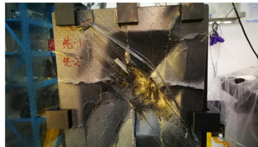
(b) The front surface of the 2 nd impact
