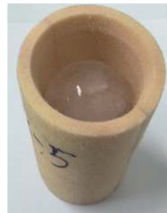
图 4 冰球弹托 Fig.4 Ice sphere with sabot
