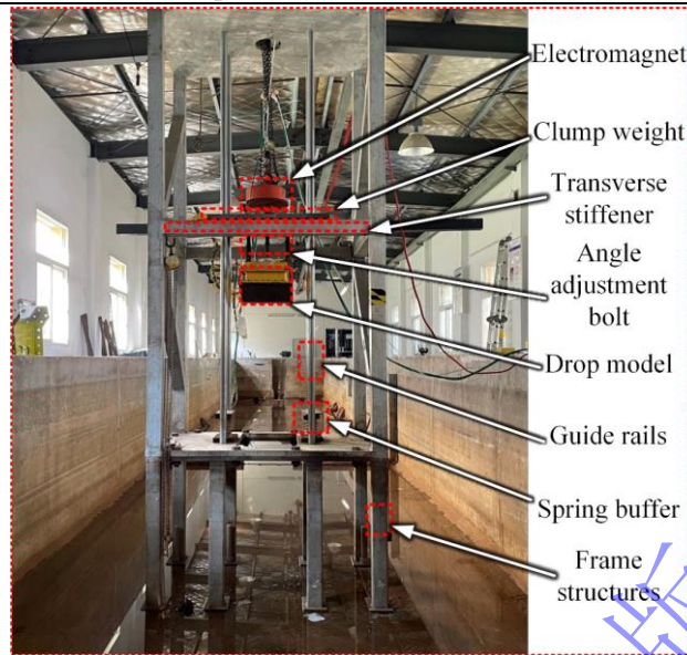
图1 入水冲击实验装置 Fig.1 Water impact experimental devices
